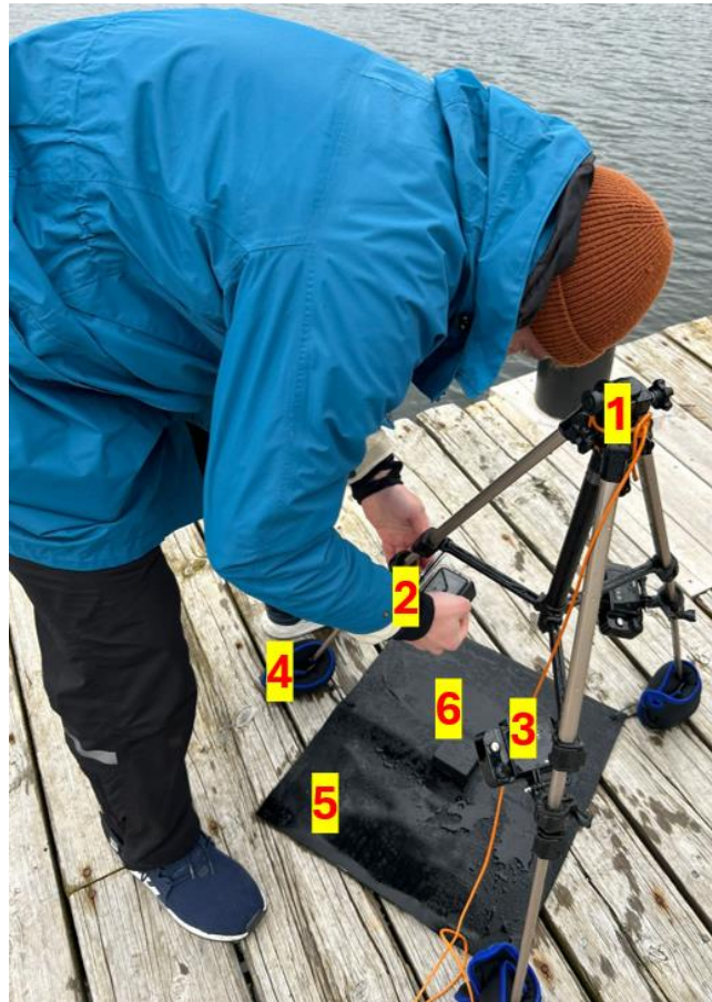
Figure 3: The components of the Low-Cost BRUV setup are as follows: 1 - camera Tripod; 2 - GoPro 9; 3 - underwater lights; 4 - ankle weights; 5 - trunk mat; 6 - bait box.
